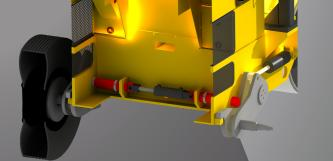
The hydraulic, auto-lock feature on the towing mechanism makes it easier and safer for the operator to attach and remove the RS206T from the tow vehicle. Once the unit is in the tow position the locking pins are put into place hydraulically from the operator's platform. The hitch is also locked in a similar fashion.
